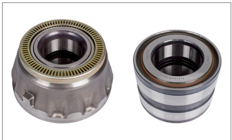
Image 1: TAM (Truck Axle Module) and THU (Truck Hub Unit)
