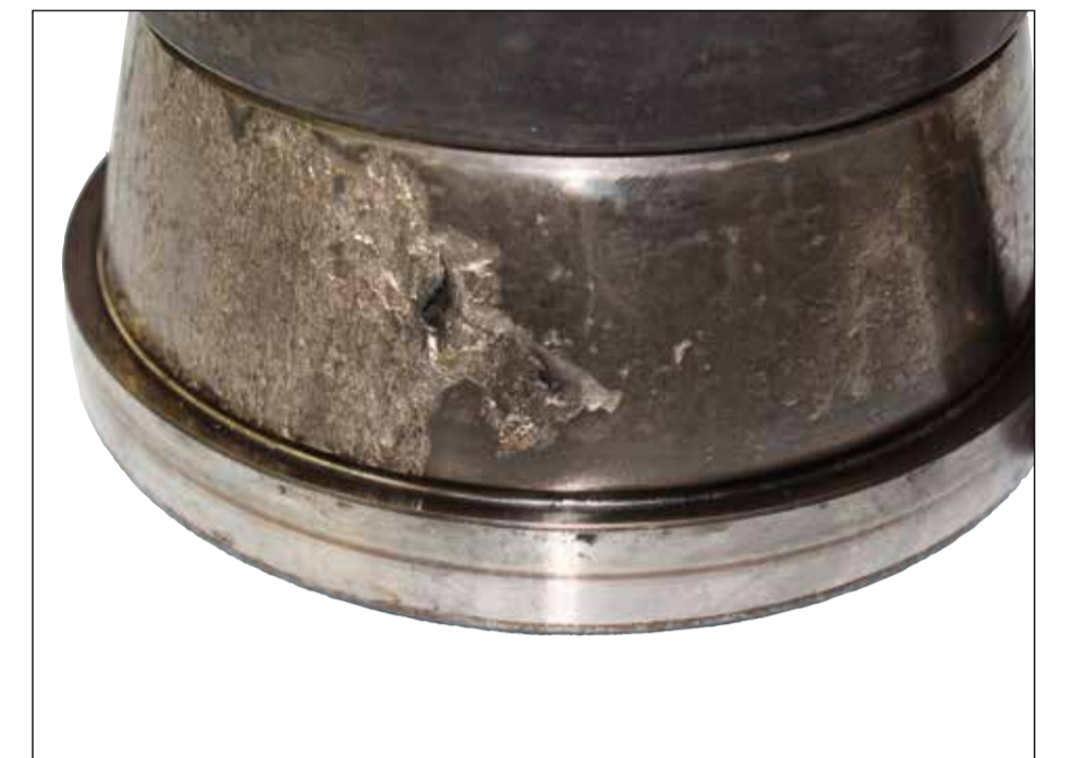
Excessive preload, overload
