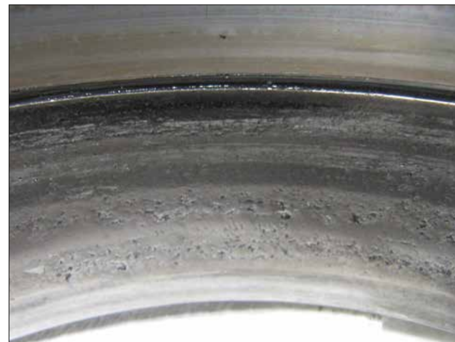
Premature wheel bearing failure
