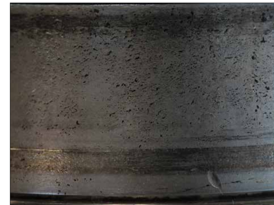
Inadequate lubrication or dirt contamination
