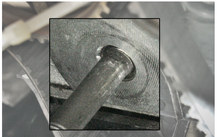
Image 2: The stud is correctly screwed in
