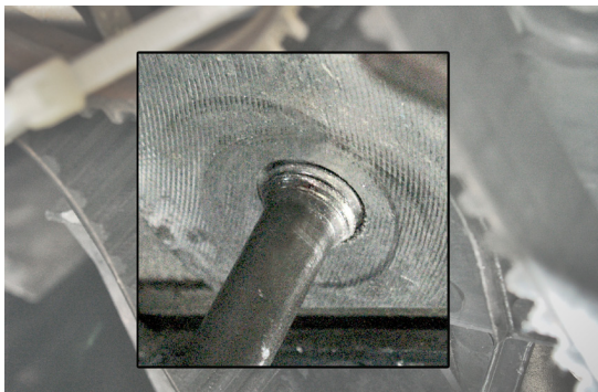
Image 1: The stud is not correctly screwed in
