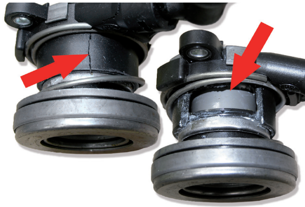
Image 5: CSC damaged by improper installation
