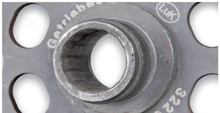
Image 2: Damaged spline profile
