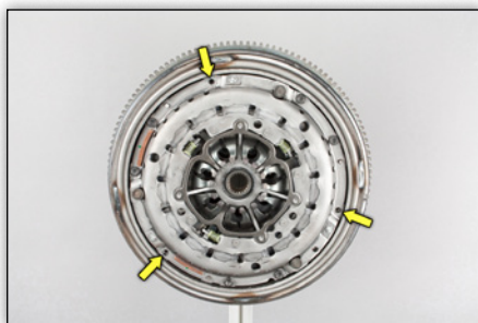
Image 9: Manually screw in the remaining 3 screws and tighten with 10.5 \pm 1 Nm
