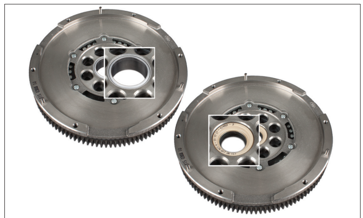
Image 1: Comparison of LuK DMF 415 0388 10 with slide bearings (left) and with ball bearings (right)
