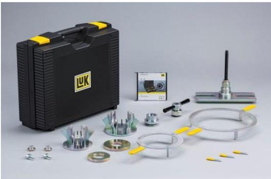
The LuK Resetting Tool Kit for Ford vehicles using the 6-speed DPS6 transmission is necessary whenever the old double clutch is used again after being removed. For example, if work was done on the gearbox gaskets and then transport lock needs to be reset again.
