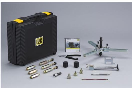
The LuK basic tool set, which forms the foundation for the modular tool system. It contains all the parts of the tool needed for all repairs of a LuK double clutch.
